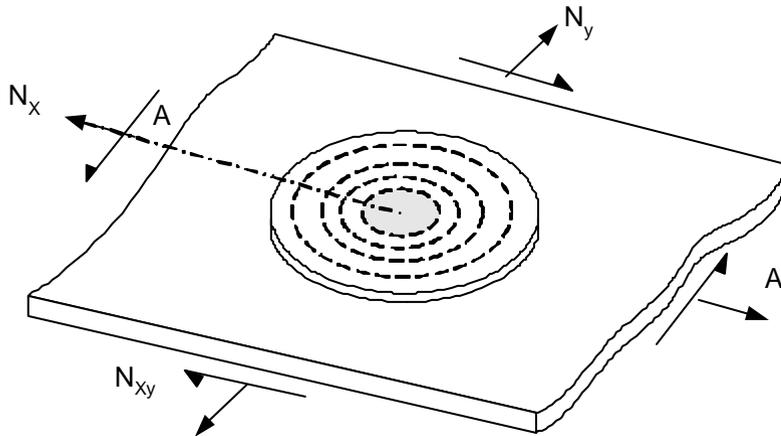
(b) 1D Analytical repair patch to a monolithic panel
